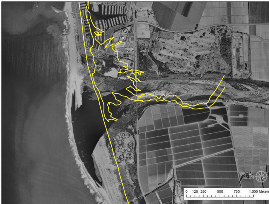
Figure 2-12. 1855 and 2005 maps of the Santa Clara River estuary. (top) The 1855 U.S. Coast and Geodetic Survey (USC&GS) map shows a meandering river channel with a broad floodplain and an extensive estuary/lagoon complex with a distributary channel network at the southern extent of the mouth complex. (bottom) The 1855 shoreline and the river mouth (and associated estuary) (yellow trace) are inland and the mouth/estuary complex is further north compared with the 2005 location.
